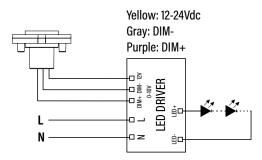
Cable Specifications: AWM 2464 22AWG 80°C 300V Length: 11.8" **CONNECTING BASE** (Pre-installed in fixture)
